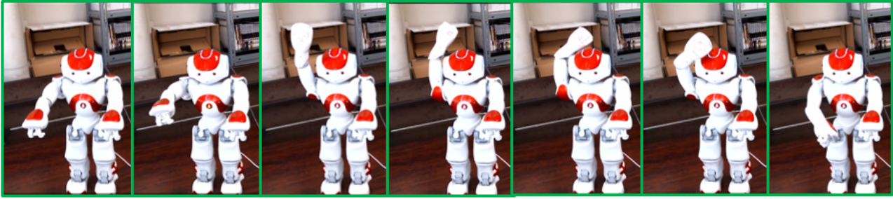
Figure 9 The state of RL-like method. The right arm is swung up to the back of the head, and the action of throwing down is executed by the real robot.
